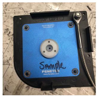
This picture shows how the cable will be attached to endcap.
